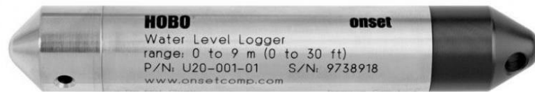
Figura 2: Sonda Onset HOB0 Water Level Logger U20-001-01.
